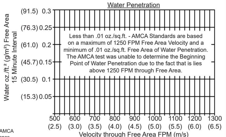
Both maximum recommended Free Area Velocity and Beginning Point of Water Penetration are 1250 FPM at standard air - .075 lbs. per cu. ft.
