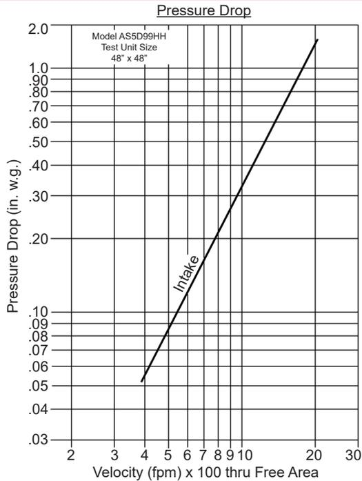
Intake air converted to standard air density.
